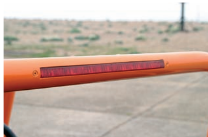
▲ Low roll bar gives this Sidewinder a wicked stance. ▼ Brake light neatly frenched into the roll-over cage. ▼ Four separate bucket seats look great. ▲ Image wheels add to the modern feel.
